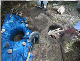
During the experiment two separate pits were dug close to the same dimensions and the water pit was lined with a standard blue tarp to keep the water from absorbing in the ground.
