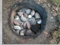
Fire pit during experiment, major fracturing occurring with discoloration.
