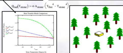
$$T_{\text{stone}}(r,t) = T_{\text{fire}} + (T_{\text{fire}} - T_{\text{ambient}}) \sum_{n=1}^{\infty} \frac{1}{n} \frac{R_{\text{stone}}}{a} \sin\left(\frac{n\pi r}{R_{\text{stone}}}\right) \frac{1}{\exp\left(\frac{n^2 \pi^2}{4R_{\text{stone}}^2} \alpha t\right) + 1}$$
